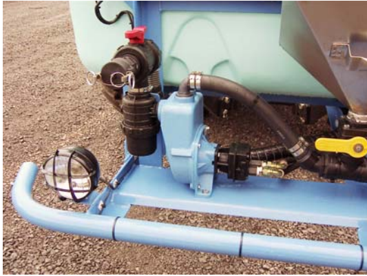
Self priming Centrifugal Pump Hydrologically driven from the tractor HYD system 400 lt/min for Filling, Agitating and Transferring
